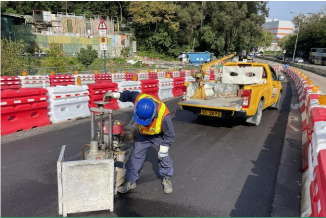
Coring of bitumen pavement sample completed on 14/11/2023
